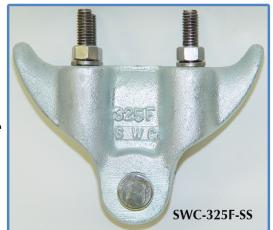
General Traffic Equipment Corp's SWC-325F is a superior strength alternative for cast aluminum clamps and with the addition of hot-dip galvanized finish, will retain corrosion resistance for many years. The SWC-325F will adapt easily to any wire entrance head or balance adjuster. The clamp accommodates up to 5/8" span wire. Standard clevis pin is 5/8" diameter.
