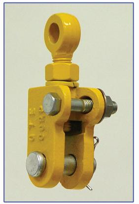
General Traffic Equipment's BALANCE ADJUSTER is one of the most useful and practical signal hardware items that has been developed. The BALANCE ADJUSTER is used on span wire and mast arm signal assemblies to assure plumbness when signal faces are not uniform. Maximum visibility is determined when signals are hung at the proper angle. A universal feature of the BALANCE ADJUSTER allows 360 degree signal indexing with a clamp to hold in any position.
